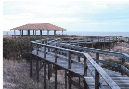
Figure 11.10: Wooden foot ramps are used to direct foot traffic through dunes in order to minimize damage to grasses and shrubs.
