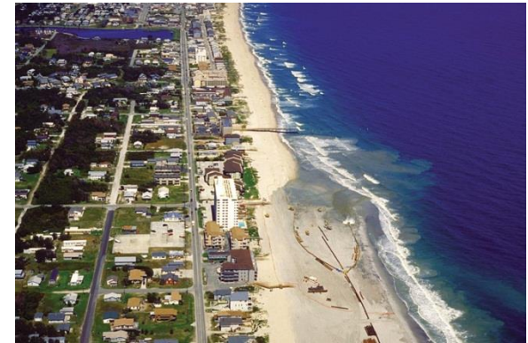
Figure 15.15: If dredge spoils offshore consist of clean sand, a means of disposing the material is to pump it to the updrift end of a beach.
