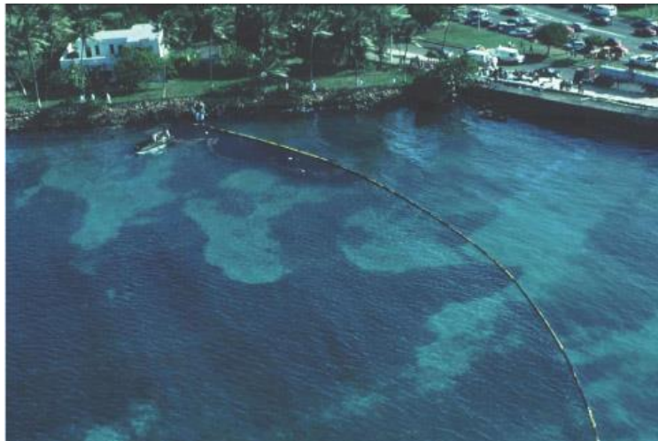
Figure 15.06a: Large, floating booms are used to contain oil slicks, the oil then being transferred to ships or barges.
